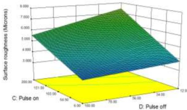
*Figure 3.21 3D plot between pulse on time and pulse off time with kerosene*
