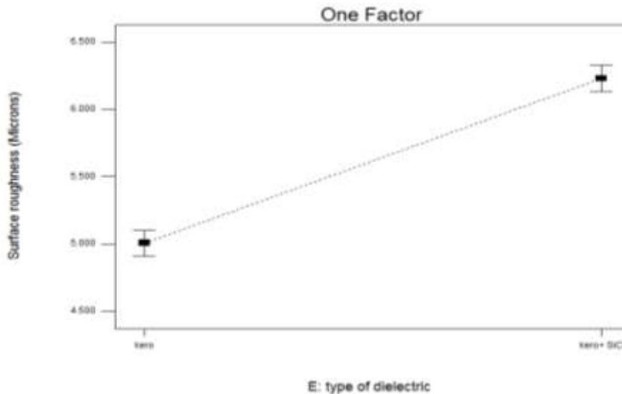
**Figure 3.13** Plot between type of dielectric medium and surface roughness at voltage(37.50 Volts), current(15.5 A), pulse off time (56 microseconds) and pulse on time(103 microseconds)
