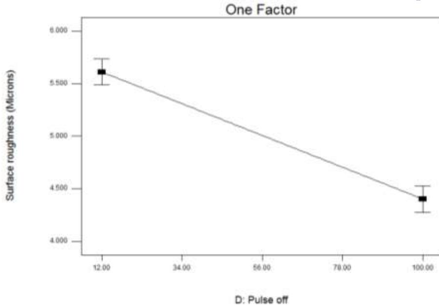
**Figure 3.11** Plot between pulse on and surface roughness at voltage (37.50 Volts), current (15.5 A) and pulse on time (103 microseconds) with kerosene
