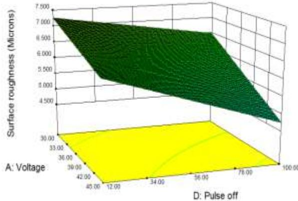
*Figure 3.20 3D plot between voltage and pulse off time with kerosene +SiC powder*
