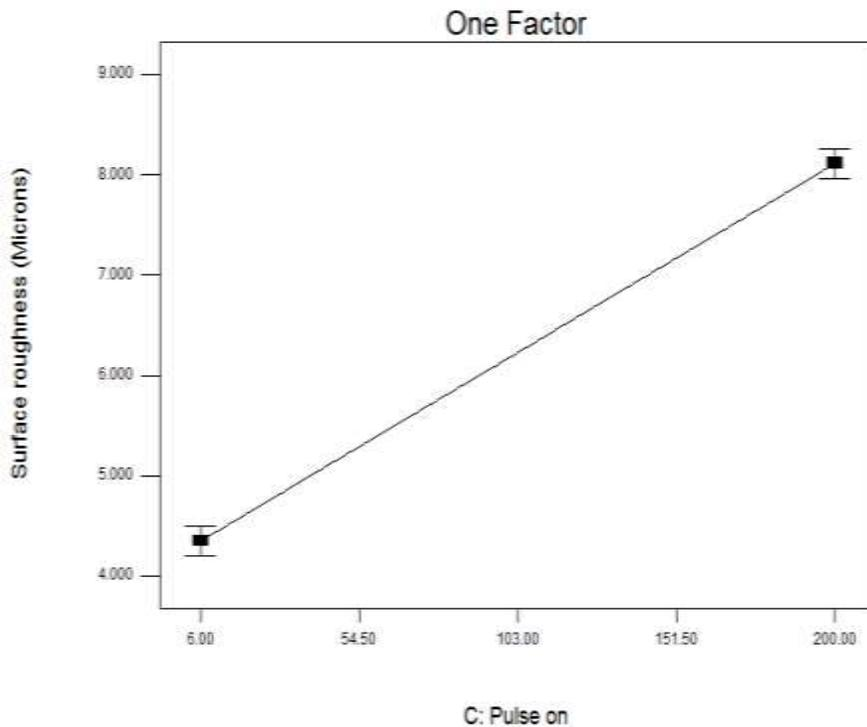
**Figure 3.10 Plot between pulse on and surface roughness at voltage (37.50 Volts), current (15.5 A) and pulse off time (56 microseconds) with kerosene + SiC powder**
