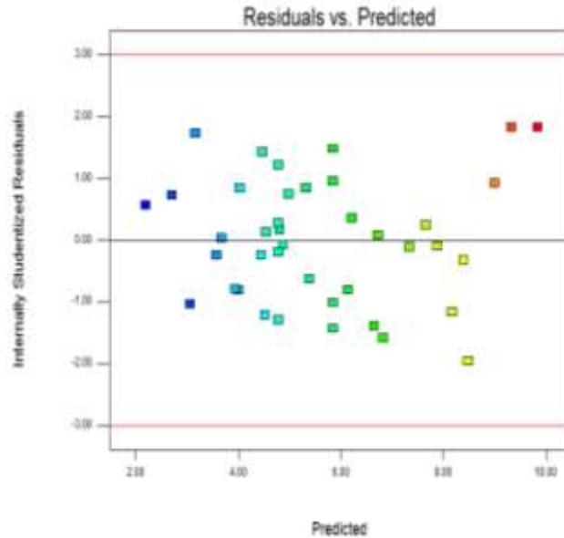
*Figure 3.2 Plot of residuals v/s predicted surface roughness*
