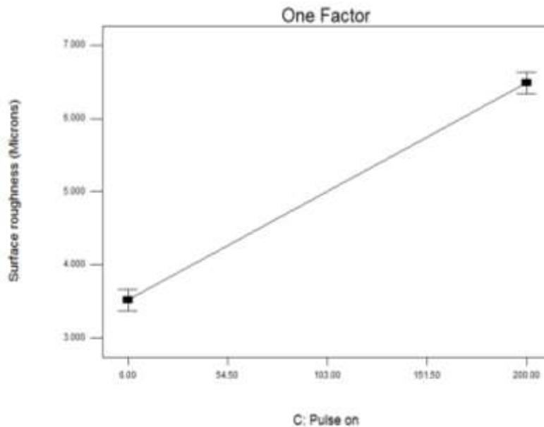
**Figure 3.9 Plot between pulse on and surface roughness at voltage (37.50 Volts), Current (15.5 A) and pulse off time (56 microseconds) with kerosene**
