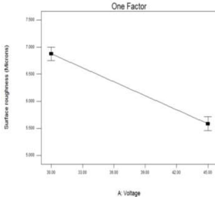
**Figure 3.6. Plot between roughness & voltage at current (15.5 A), pulse on time (103 microseconds) pulse off time (56 microseconds) with kerosene +SiC powder**
