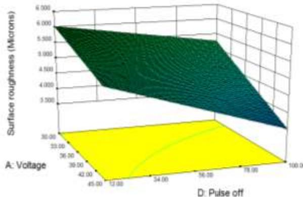
**Figure 3.19 3D plot between voltage and pulse off time with kerosene**
