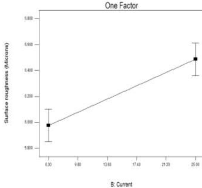
**Figure 3.8 Plot between current and surface roughness at voltage (37.50 Volts) Pulse on time (103 microseconds) and pulse off time (56 microseconds) with kerosene +SiC powder**
