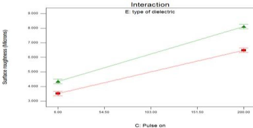
**Figure 3.18 Interaction plot between type of dielectric medium and pulse on time for surface roughness at constant voltage 37.5 V, constant pulse off time 56 microsecond and constant current 15.5 A**
