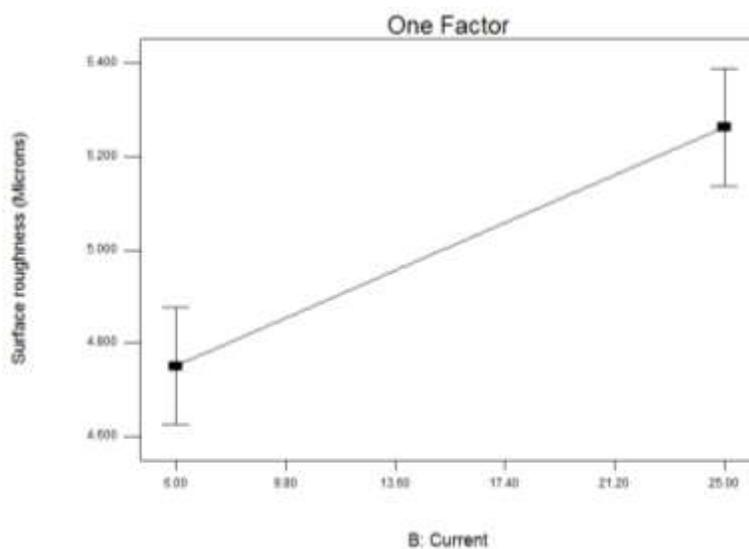
**Figure 3.7 Plot between current and surface roughness at voltage (37.50 Volts), pulse on time (103 microseconds) and pulse off time (56 microseconds) with kerosene**
