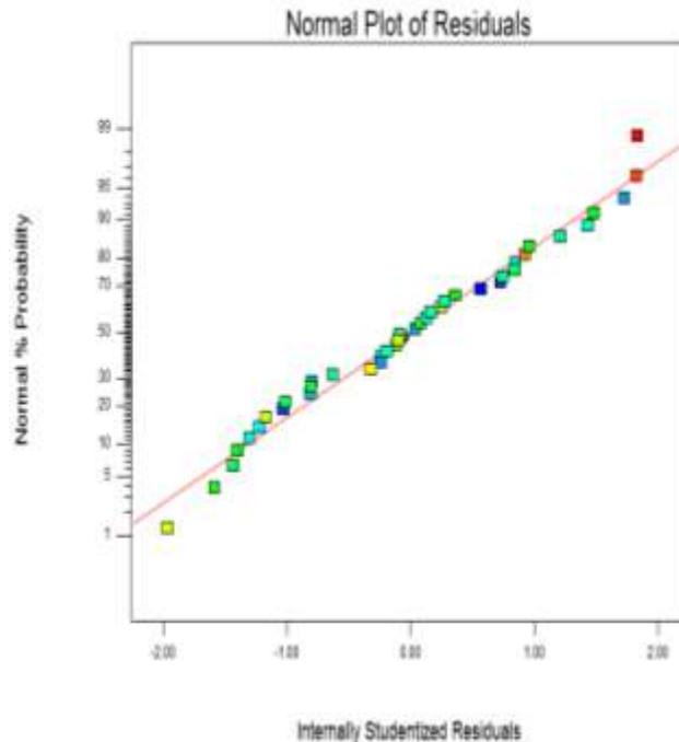
**Figure 3.1 Normal probability plot of residuals for surface roughness**
