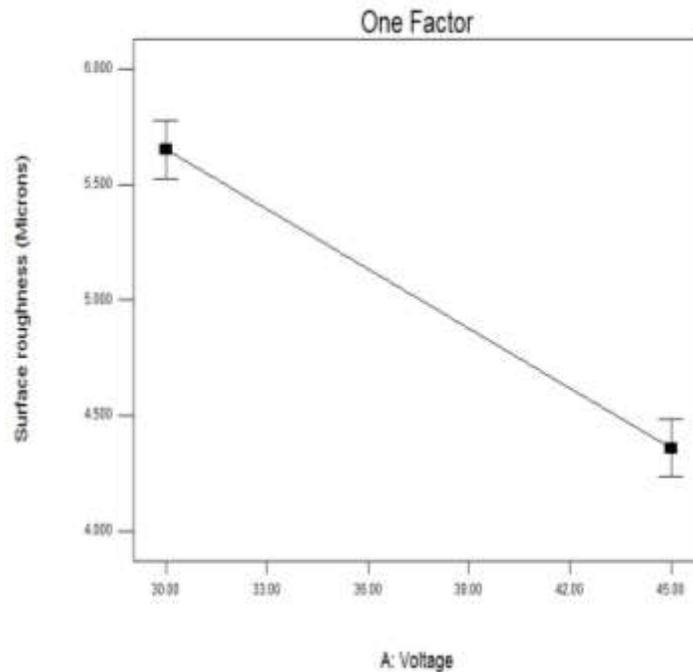
Figure 3.5. Plot between roughness & voltage at current (15.5 A), pulse on time (103 microseconds) and pulse off time (56 microseconds) with kerosene
