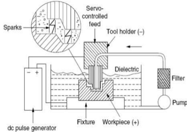
**Figure 1.1 Schematic diagram of EDM Components**
