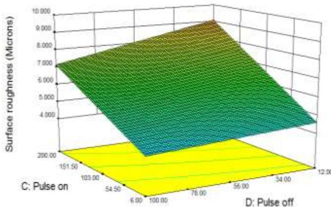
*Figure 3.22 3D plot between pulse on time and pulse off time with kerosene +SiC*
