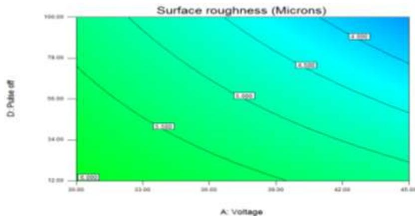
**Figure 3.14** Contour plot between voltage and pulse off time for surface roughness at constant current 15.5 A and pulse on time 103 microsecond with kerosene
