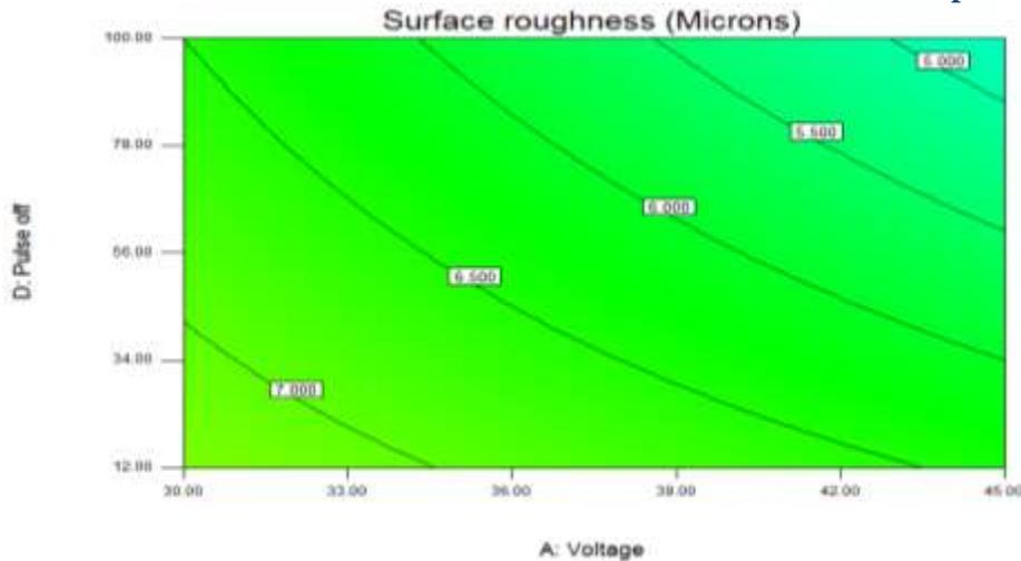
**Figure 3.15** Contour plot between voltage and pulse off time for surface roughness At constant current 15.5 A and pulse on time 103 microsecond with kerosene + SiC Powder
